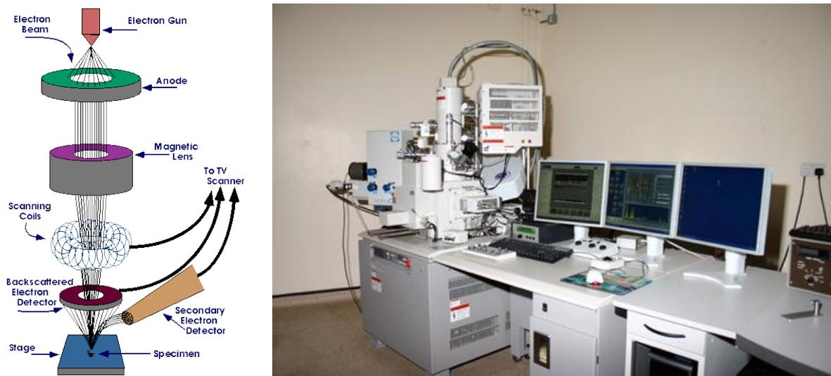
Figure 15: Schematic drawing (Purdue University) of the working principle of a SEM and the used SEM setup at Durham University ([www.dur.ac.uk](http://www.dur.ac.uk)).
