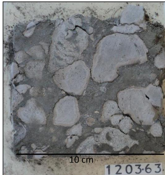
Fig.4) Slab cored section from F02-03 well (depth in meters is indicated below core). Sediment of Mid Miocene Unconformity, consisting of a conglomerate of limestone & sandstone clasts in a clay matrix. The green color is related to the glauconitic content
