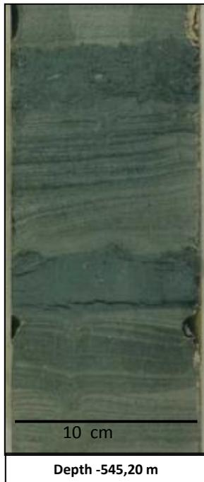
Fig.3) Core section from B13-03 well. Sediment of Upper North Sea group, consisting of alternating sandstone beds and claystone layers (photo from NLOG website)
