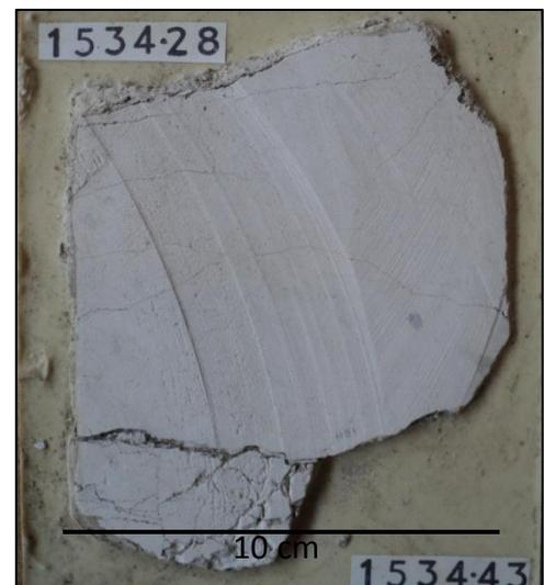
Fig.6) Slab cored section from F02-03 well (depth in meters is indicated below core). Sediment of the Late Cretaceous chalk group is composed of homogeneous bioclastic chalk.
