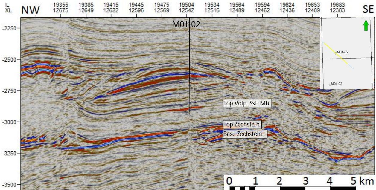
Figure 37 - Seismic section through the M1-A field in the south of the M1 block. A high red reflector (trough) indicates the Volpriehausen Sandstone reservoir.
