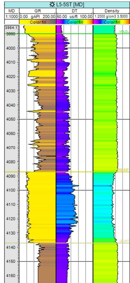
Figure 36 - Well log of well L5-5 (st) in the L5-FA field, showing a 50 m thick Volpriehausen Sandstone reservoir, with clay-siltstones above and below.
