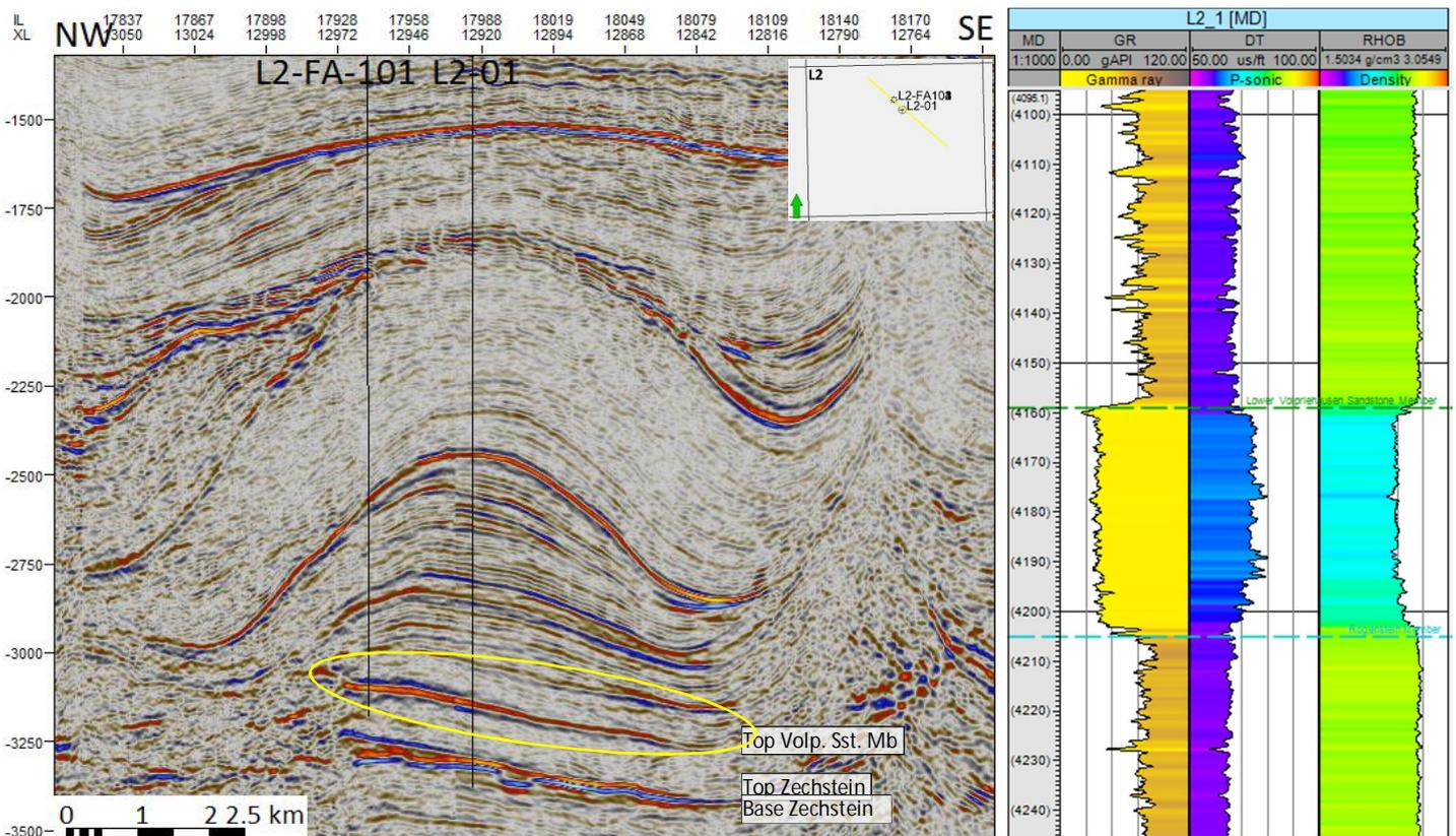
Figure 33 - Seismic section through the L2-FA field, showing the locations of the L2-FA-101 and L2-01 wells. The Top Volpriehausen is a peak with a strong trough below and a less high peak below that.
