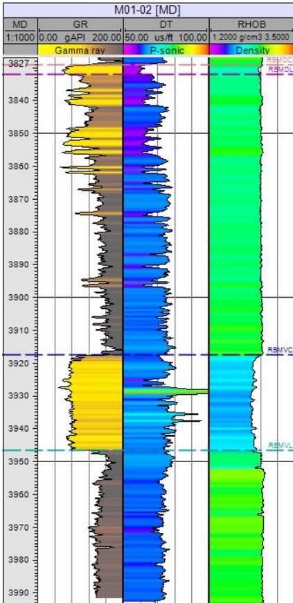
Figure 39 - Well log of well M01-02 in the M1-A field, showing a 30 m thick Volpriehausen Sandstone reservoir. Clay and siltstones are present below and above the Sandstone Member. Questionable if the peak in DT at 3928 m is correct or a measurement error.
