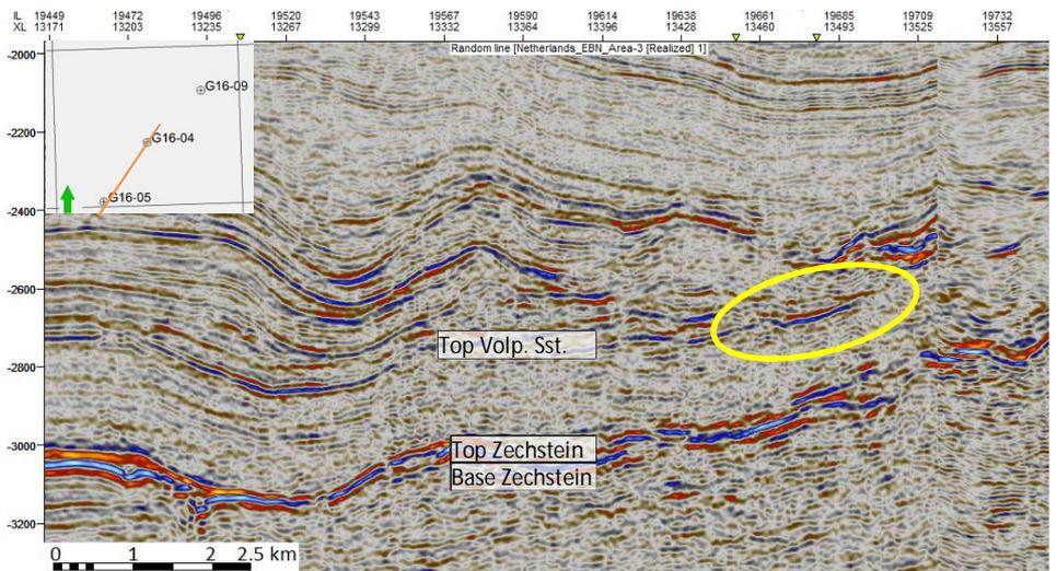
Figure 40 - Seismic section through G16-B. The field is indicated with the yellow circle, the location of the seismic section is indicated in the map view of the G16 block in the upper left corner.
