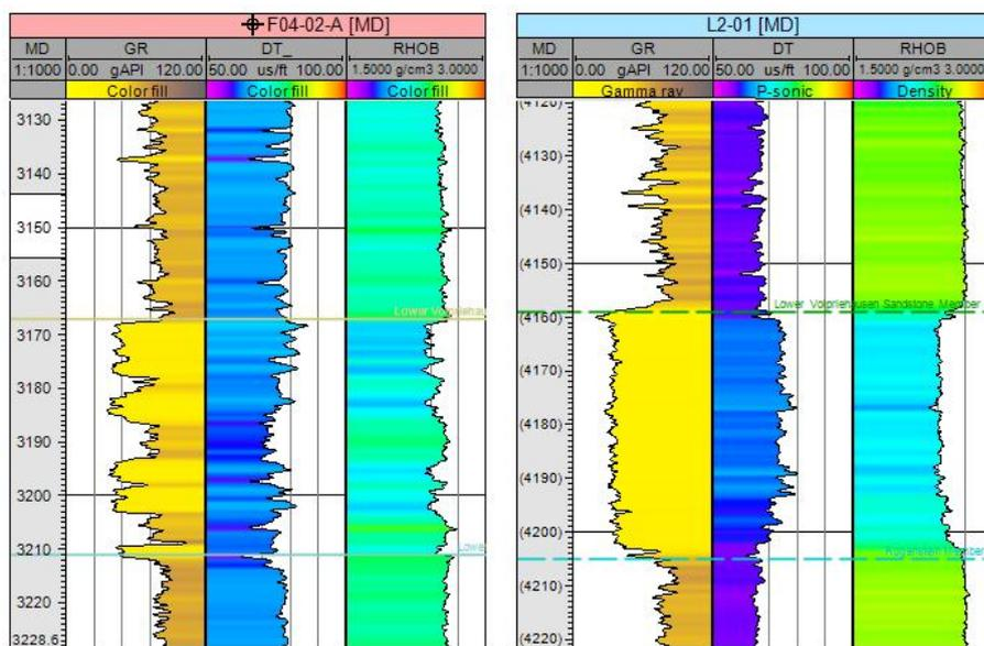
Figure 45 - Well logs of the Volpriehausen Sandstone Member of a dry well in the study area (F04-02-A) and a well of a gas field outside the study area (L2-01).
