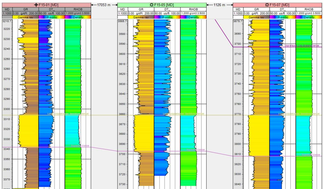
Figure 30 - Well logs of exploration wells near the F15-A field showing the top and base of the Volpriehausen Sandstone Member. The GR logs show massive sands with low clay-content. The RHOB log also shows a clear distinction between the over- and underlying claystone members, and the Sandstone member. The DT log shows an overall decrease in porosity within the Sandstone Member, towards the base.
