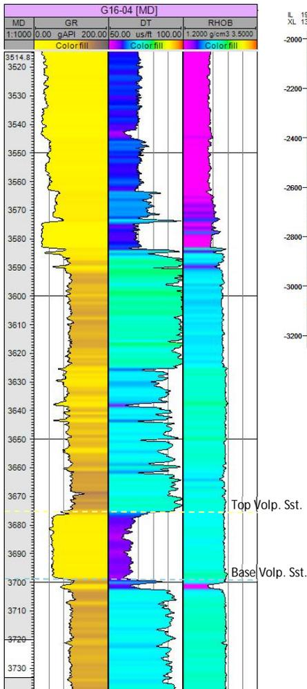
Figure 41 - Well log of G16-04. The Volpriehausen Sandstone member is located at a depth of -3675 to -3699 m. The sandstone member is clearly distinguishable on the DT log, but not on the RHOB.
