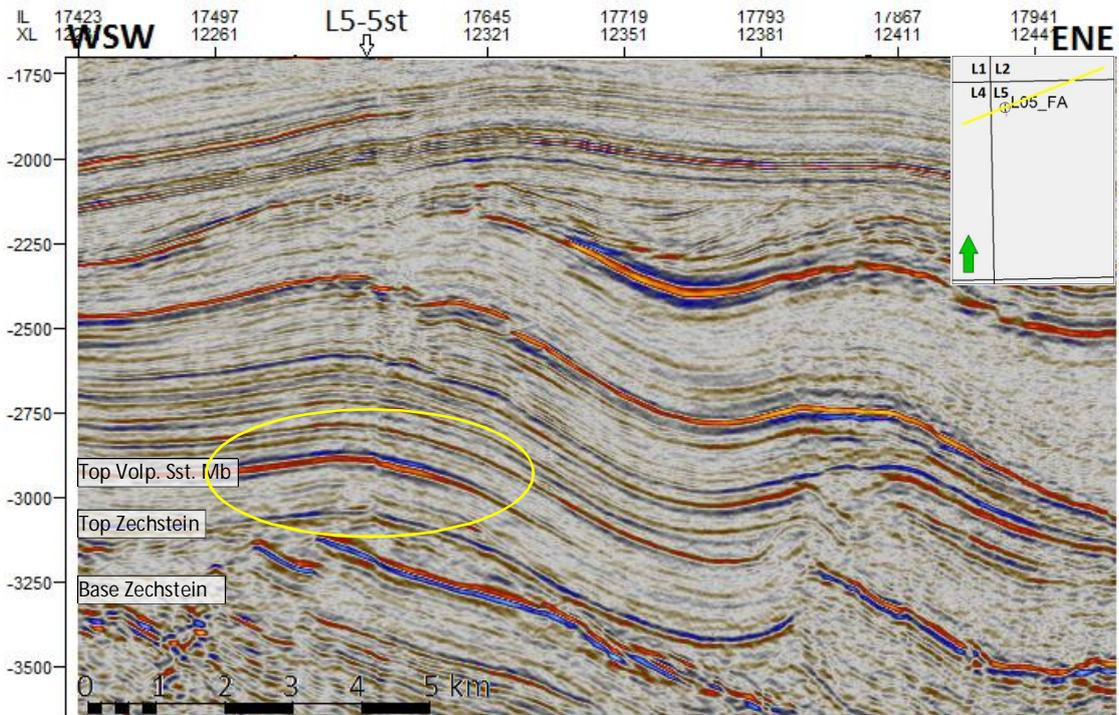
Figure 35 - Seismic section through the L5-FA field in the northwestern corner of the L5 block, showing the location of the L5-5st well (Figure 36). The Top Volpriehausen Sandstone Member can be recognized by a high blue (peak) reflector, with a high red (trough) reflector below. The faulted Zechstein below has provided a migration path for the gas.
