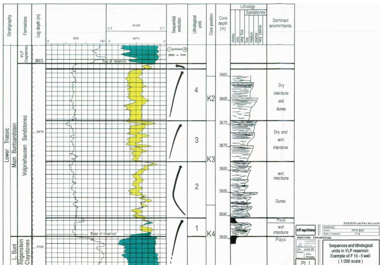
Figure 5 - Lithological units within the Volpriehausen Sandstone Member based on core data from F15-5 and F15-7 wells. From: Vittori et al., 1990.
