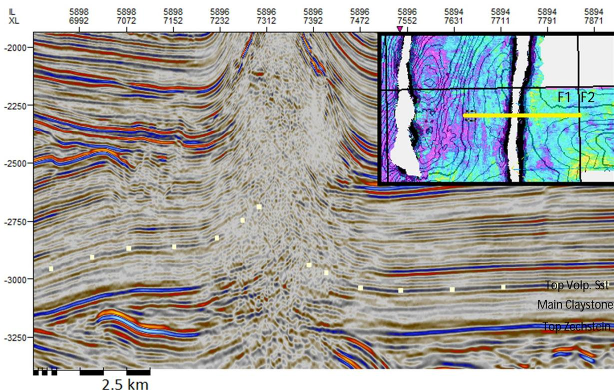
Figure 7 - Seismic section in the north of the study area showing the typical seismic character of the Volpriehausen and its underlying lithologies, as well as the decreased seismic signal near salt domes. The yellow dots indicate the interpreted Top Volpriehausen Sandstone Member. In the upper right corner an overview map (maximum amplitude in window of 10 ms above and below the interpretation) shows the location of the seismic section with a yellow line.
