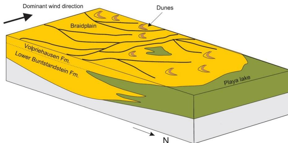
Figure 4 – Depositional model for the lower Buntsandstein and Volpriehausen formations in the Dutch offshore. Yellow = predominantly sandstones, green = predominantly siltstones. During deposition of the Volpriehausen Formation fluvial systems built out to the north, resulting in thinning sandstones and an increasing clay-content towards the north. Modified after: Wong et al. (eds) 2007.
