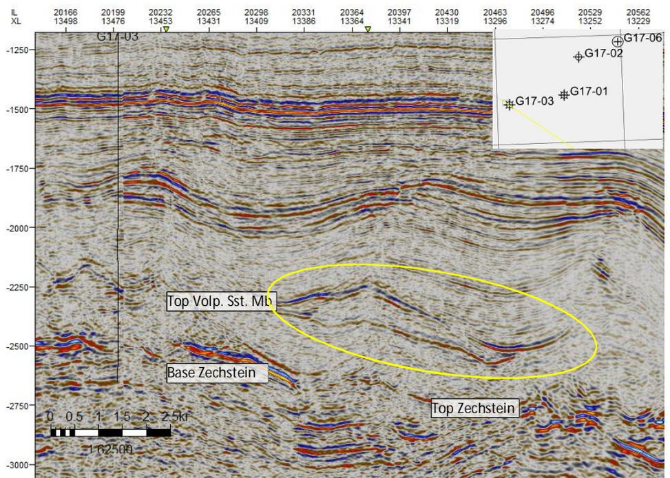
Figure 44 - Seismic section through the G17 block. The location of well G17-02 is indicated. The Top Volpriehausen Sandstone Member is characterized by a trough, with a high peak and less high trough below.
