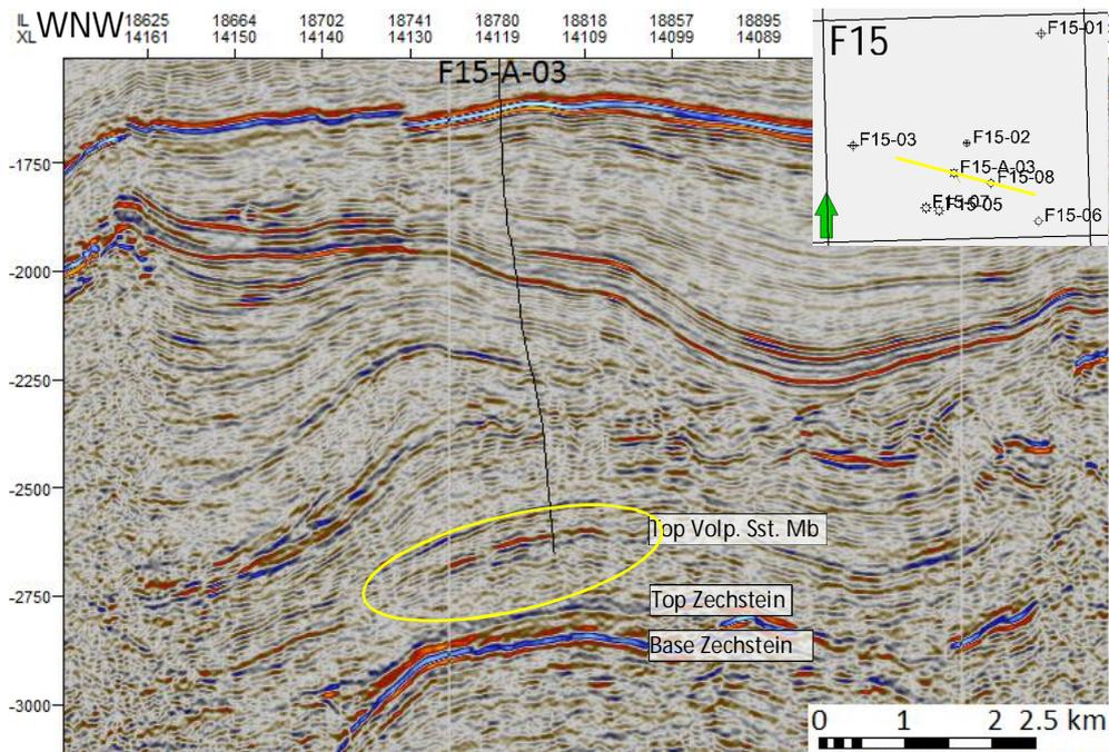
Figure 31 - Seismic section showing the turtle-back anticline structure of the F15-A field. The Top Volpriehausen Sandstone Member is characterized by a strong red reflector, which is a trough, with a peak (blue reflector) below.
