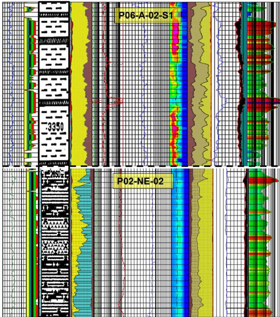
Figure 7. NuTech model results for the Muschelkalk in P06-A-02-S1 and P02-NE-02. Both lithology and pay were misinterpreted by NuTech. It appears that resistivity played a key role in both lithology and pay determination.
