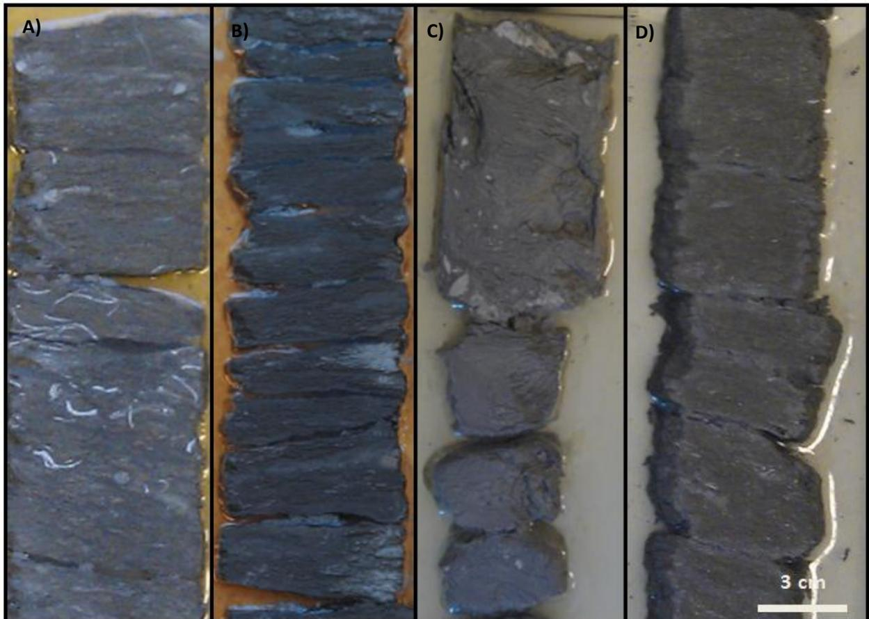
**Figure 23 (above).** Offshore facies in core. A) Grey/brown silty marls with shell debris bed and pyrite concretions (AND-04 1496m MD). B) Dark grey/brown laminated silty marls (AND-04 1504m MD). C) Grey/brown massive marl with calcite concretions/intraclasts (AND-03-S2 1190m MD). D) Grey, massive marl, slightly silty (AND-03-S2 1248m MD).
