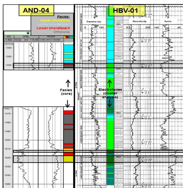
Figure 27. Core-log calibration using *k*-Means Clustering. Interpreted core facies (left) are calibrated to gamma ray, resistivity and sonic log data of HBV-01 (right). The best fit was obtained for 4 clusters.
