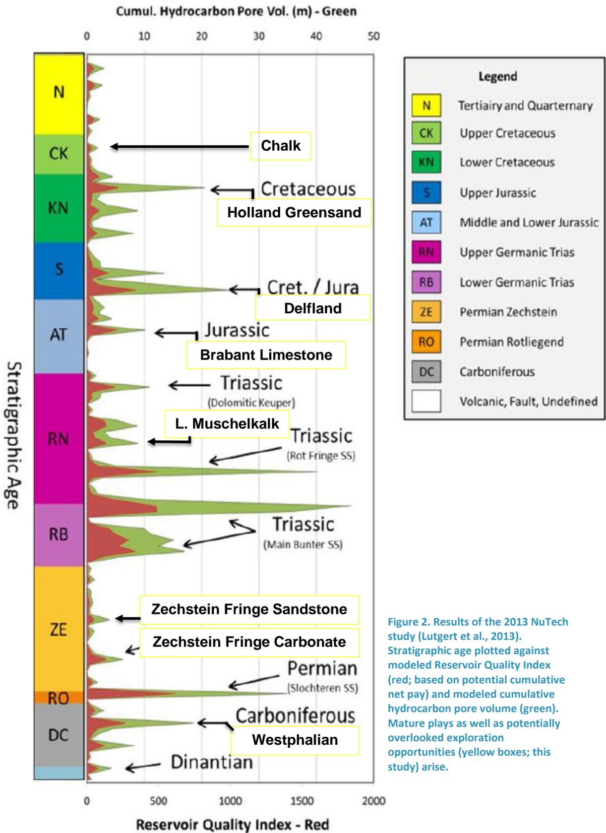
Figure 2. Results of the 2013 NuTech study (Lutgert et al., 2013). Stratigraphic age plotted against modeled Reservoir Quality Index (red; based on potential cumulative net pay) and modeled cumulative hydrocarbon pore volume (green). Mature plays as well as potentially overlooked exploration opportunities (yellow boxes; this study) arise.
