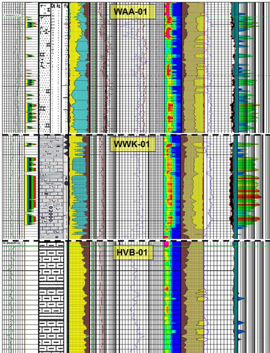
Figure 4. Modeled NuTech results and composite log lithology for WAA-01, WWK-01 and HVB-01. The three wells represent the varied interpretations by NuTech for this formation.
