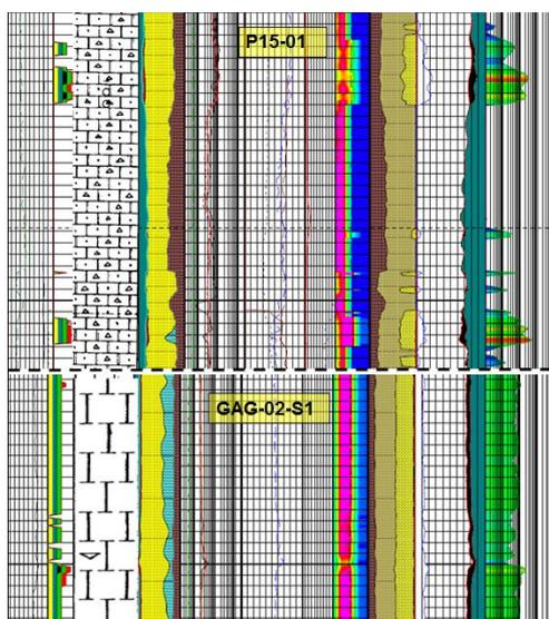
Figure 1. NuTech log interpretation and mud log lithology. Small amounts of potential net pay have been modeled by NuTech, whereas in reality, the formation is completely dry from mud logs.
