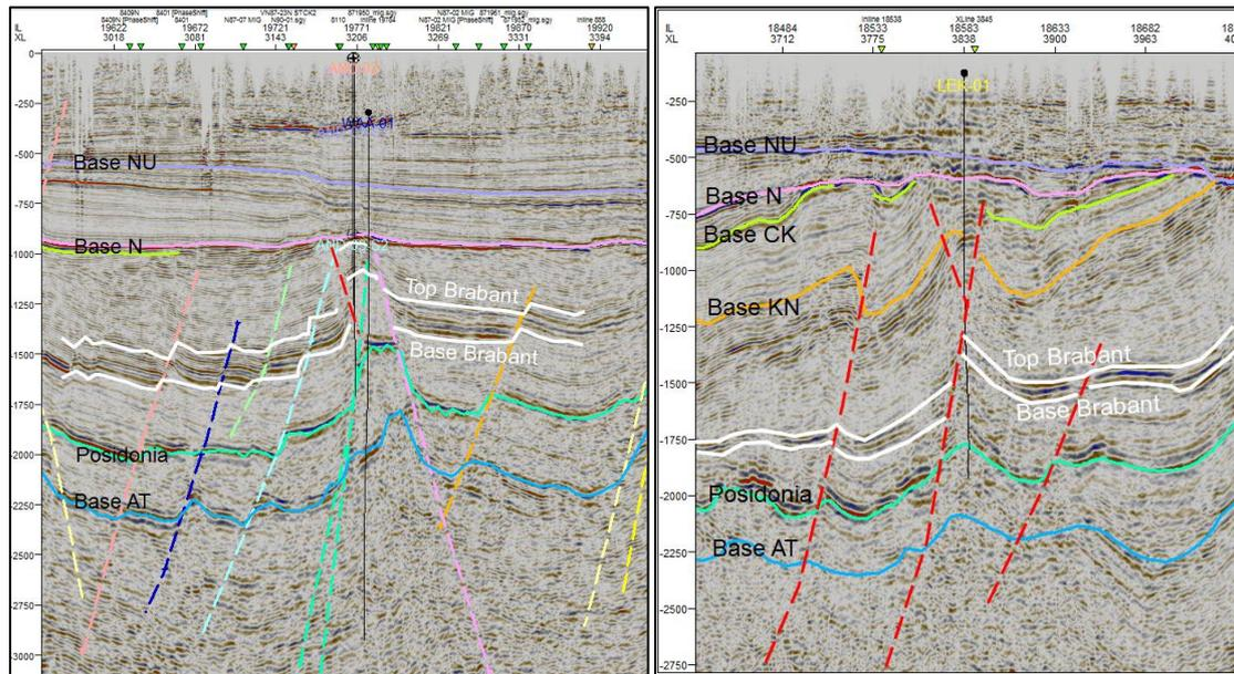
**Figure 6.** A) SW-NE seismic line (random line 3D Terracube onshore) over the Andel stranded field. The inversion trap contains oil in stacked reservoirs (SLDN, ATBR, ATWDM). B) SW-NE seismic line (3D Terracube onshore) over the Lekkerkerk stranded field, showing the fault-dip closure at Brabant level. Faults by Van Der Kroef (2014). See text for details, for location see Figure 5.
